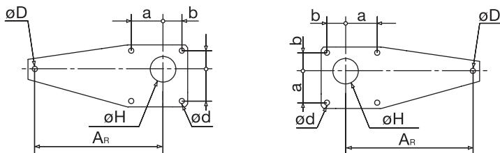
**Table 3.12 Hyponic® Torque Arm Recommended Dimensions (in.)<sup>[1]</sup>**
