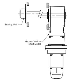
**Incorrect:** Poor concentricity of driven shaft and mounting flange
