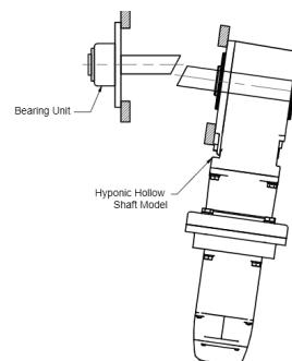
**Incorrect:** Poor perpendicularity of driven shaft center and mounting flange surface
