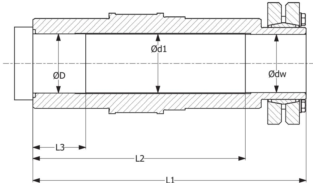
Recommendations for the design of the driven shaft if Shrink Disc connection method is selected:
