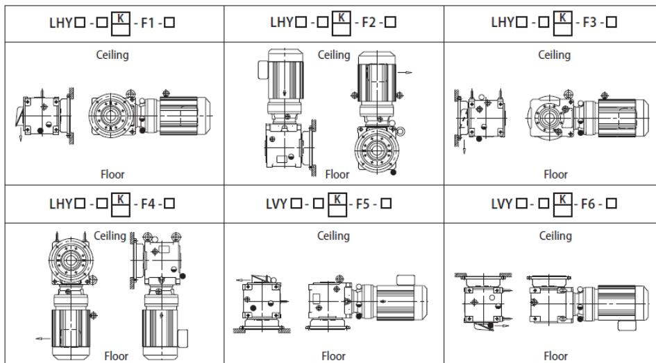
**Fig. 2.21 Keyed Hollow Output Bore – Output Flange Right**
