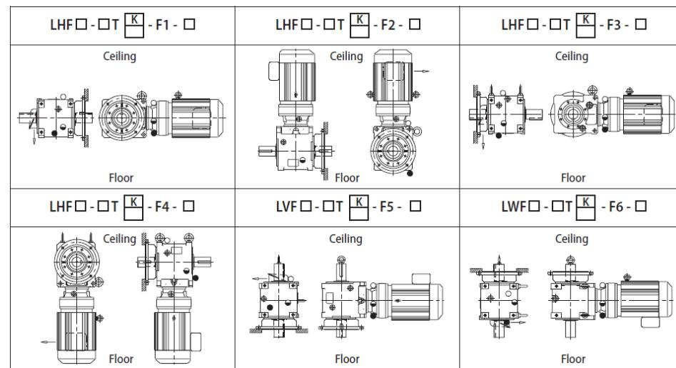
**Fig. 2.25 Double Extended Solid Output Shaft (T) - Output Flange Right**
