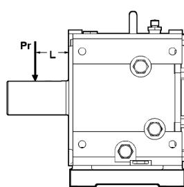
Pr from table must be  $\geq$  Pr
