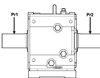
For double extension, Pr1 and Pr2 is assumed to be in the same direction. Pr0 from table must be  $\geq$  Pr1+ Pr2
