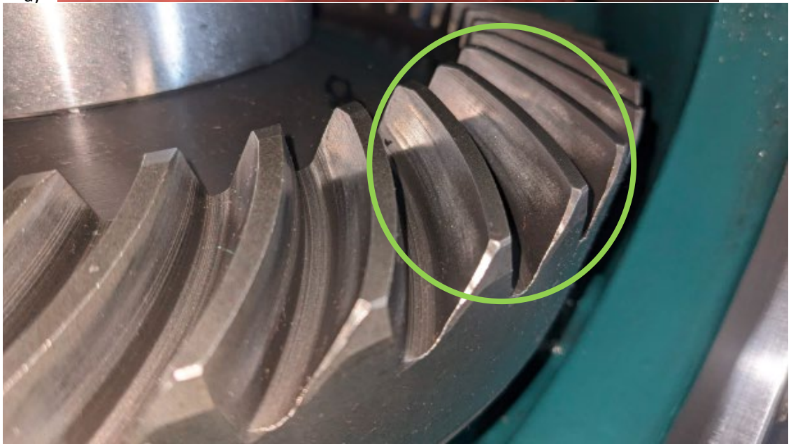
Figure 10: Bevel gear set condition. a) bevel pinion shows mild polishing. b) bevel gear shows mild polishing.
