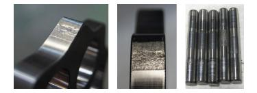
Lubrication failure is the most common limitation on Cyclo<sup>®</sup> life.
