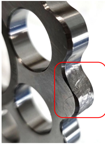
Figure 4: "Damaged" cycloidal disc with a simulated 'worn-out' lobe (highlighted)- This was achieved by removing material from the lobe flank and increasing the surface roughness.
