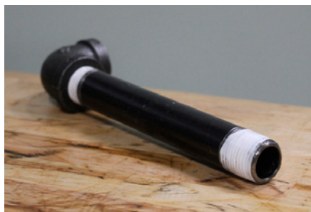
Figure 1—Typical threaded pipe connection with thread sealant.
