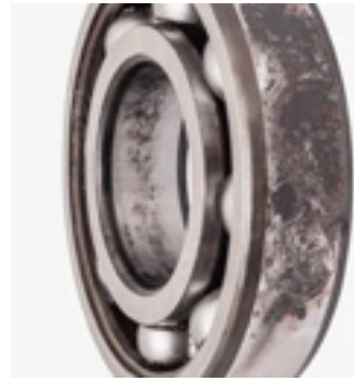
Outer ring slippage caused by improper housing fits.
