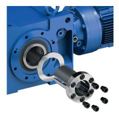
The patented Sumitomo Taper-Grip® bushing system enhances the Cyclo® BBB4 value by offering a simple shaft-mounting device that provides selfaligning, backlash-free torque transmission to the driven shaft.
