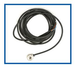
Vibration sensor – The vibration sensor is a MEMS type sensor that comes with a 3m length of cable with a field Wireable connector to allow for easy installation in the field. The sensor mounts to the application using 1 M5x20 bolt. Max Qty - 4
