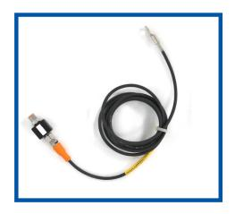
Temperature sensor – The temperature RTD is used for constant temperature monitoring of any component. It delivers a 4-20ma signal that is recorded for future reference allows for 2 alarm levels per temperature channel. Max Qty - 2
