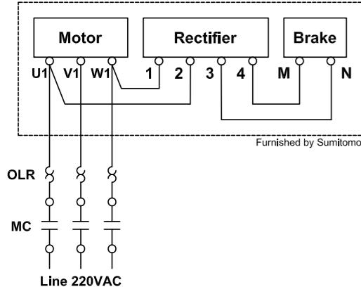
Normal Brake Action, 380V Motor, 220V Brake, Tapped
