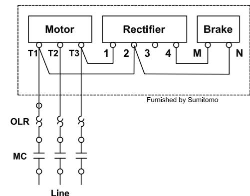
Fast Brake Action, 460V or 575V Brake
