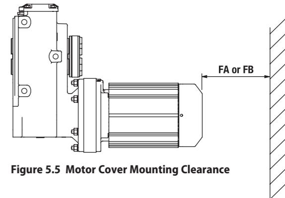
Figure 5.5 Motor Cover Mounting Clearance
