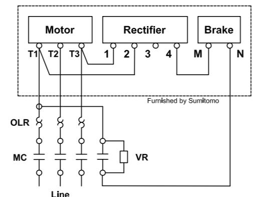
**Brakemotor Inverter Wiring Connection, EP.NA Motor****Models FB-01A1 through FB-15E, 230/460V, 60Hz or 575V, 60Hz**
