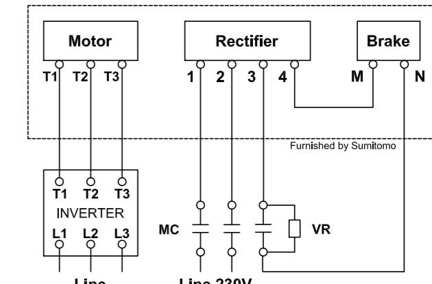
Fast Brake Action, 460V or 575V Brake
