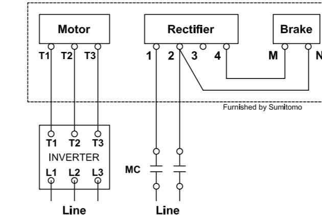
Fast Brake Action, 230V Brake
