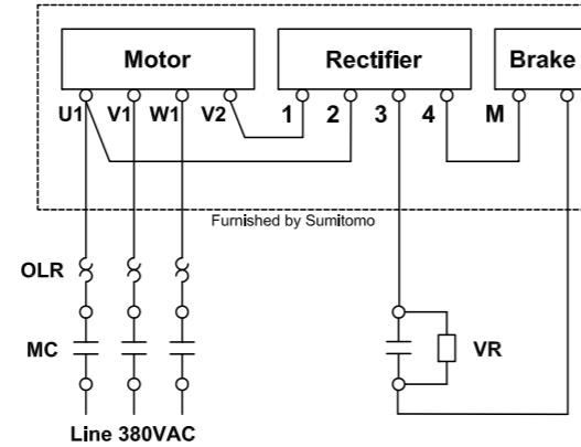
Fast Brake Action, 380V Motor, 220V Brake, Separated
