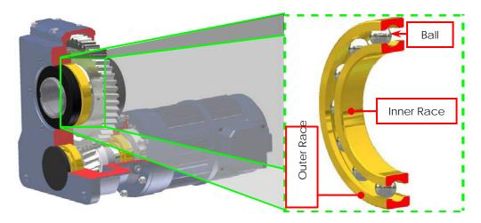
As noted, a bearing is a <u>low-friction</u> device, it is not friction-free. As one race rotates about the other race, the balls (or rollers) likewise rotate/slide within the race. The rotating/sliding action of the balls (or rollers) creates friction between these bearing components thereby creating an additional avenue for energy loss.
