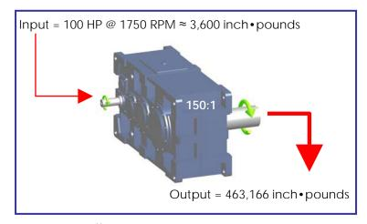
If this speed reducer were 100% efficient, it would be concluded that the 3,600 in•lbs of torque being applied to the input shaft would generate 540,000 in•lbs of torque at
