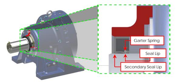
Since these seal lip(s) are riding against a rotating shaft (or collar), friction at this interface is developed, hence, an energy loss (albeit small) is realized. The amount of this energy loss due to friction is dependent upon many factors that include shaft speed, shaft diameter, and the surface finish/roughness against which
