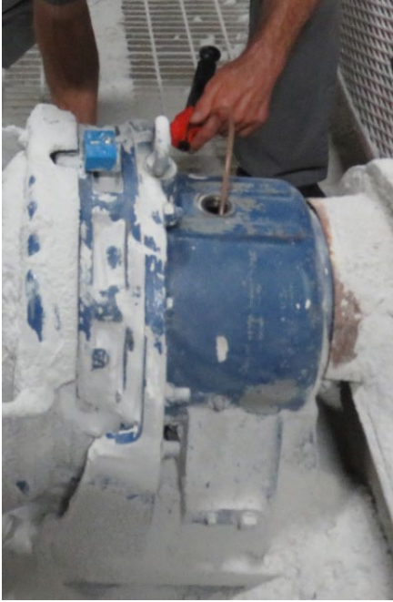
Figure 1: Oil sampling on in-line gearbox.
