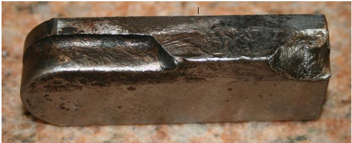
Damaged Paramax Speed Reducer Key
