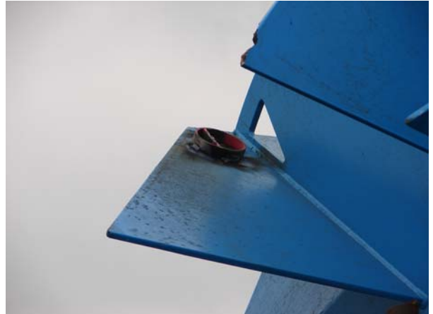
Figure 9. Added Weight to Re-Balace Aerator 1
