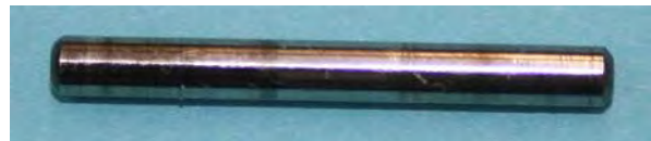
Figure 23. Micropitting of the ring gear pins
