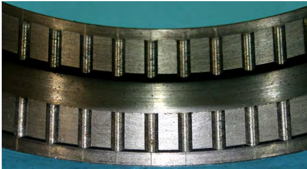
Figure 24. Mild abrasion in the ring gear pin bores
